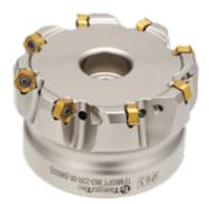
The PTKU inserts are a double-sided ten cutting edge line specifically dedicated to high feed machining. They are available in two sizes: 05 mm and 10 mm. The new inserts have a maximum cutting depth of 1.5 mm and 3.0 mm, respectively. The PTKU line covers a wide industrial range including mold and die and general engineering applications.
